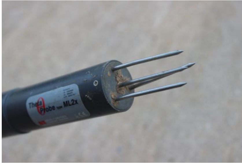
Figure 4.5. Photographs of theta probe used to measure initial moisture content of the soil at each site before infiltration testing was performed.
