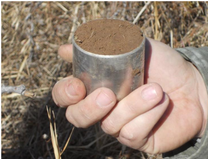
Figure 4.6. Bulk density sample collected in the field from the Oakland-Zion site.
